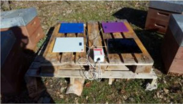
If the bottom of your hives is made from plastic Nicot, you will need to install an adaptor (the hive scale-plates measure 30x30 and are therefore adapted either to small hives such as Warré types or larger hives with a solid wooden base. If the hive base is flexible, you will need to add a 45x45 tile as reinforcement). You will also need to place a tile under the plate to obtain a better signal.
